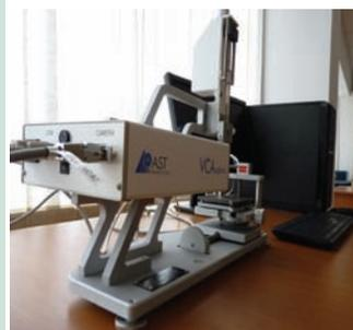
Fig. 53. Contact angle measurement machine apparatus
