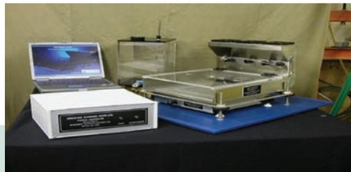
Fig. 51. Echipament "sweating guarded hotplate thermal controller"
